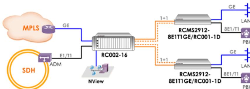
RCMS2912 series connected in pairs to extend 8 x E1/T1 and GE over 1+1 redundant fiber links
