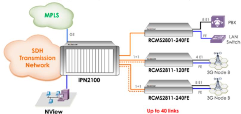
**Multi-service cards working with remote RCMS to deliver 1-8 E1s and aggregate wire-speed Fast Ethernet into Metro Ethernet/IP transportation**
