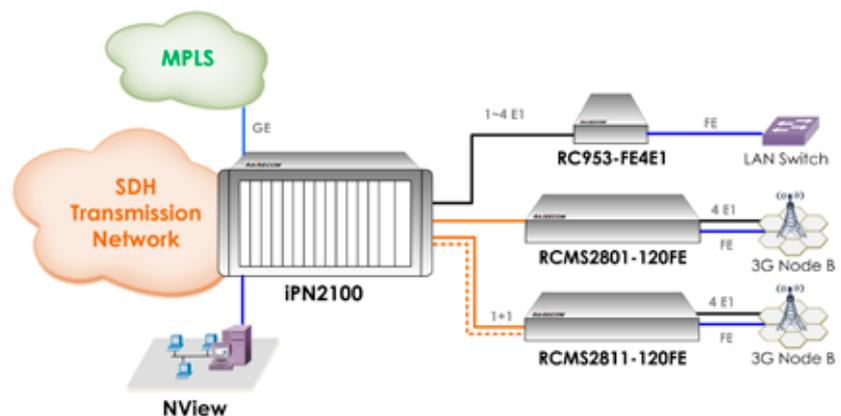
iPN2100-PTU-4GE switches and aggregates tributary Ethernet services to Metro Ethernet backbone
