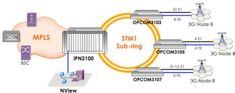
IPN2100 MSAP provides Mobile Backhaul through multiple STM-1 sub-rings, transmitting voice and data traffic on E1 and Fast-Ethernet simultaneously
