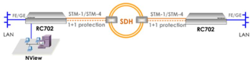
Delivering point-to-point Ethernet services over STM-1/STM-4 circuits with 1+1 protection
