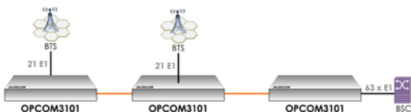
OPCOM3101 deployed as an Add & Drop Multiplexer (ADM) in a daisy chain
