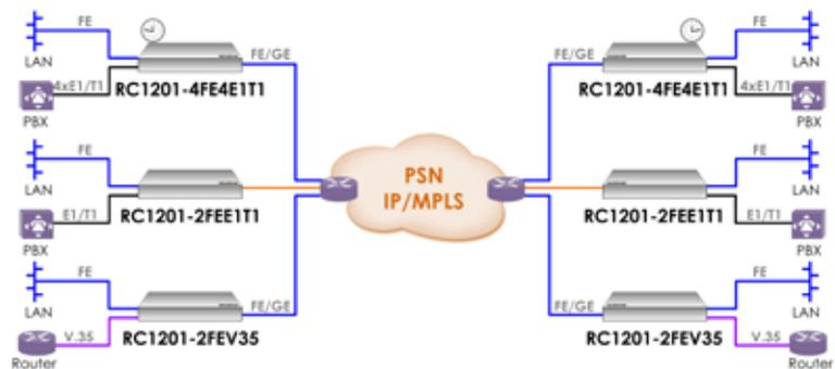
Point-to-point application, connecting E1 and V35 across packet-switched networks
