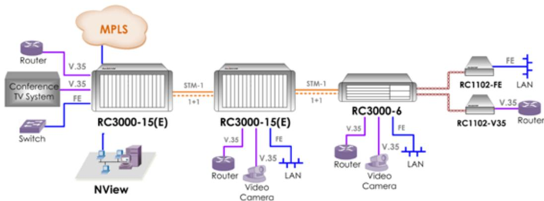
High-speed data application of Multi-Service Access Node
