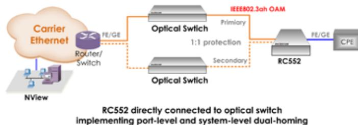
RC552-FE(Rev.B) and RC552-GE(Rev.D) continue the modular design of Raisecom media converters and the OAM features of RC552 series. Fiber uplink protection, layer-2 switching functions and web management makes the media converter a powerful Ethernet access device in a carrier's network supporting multi-service access.
