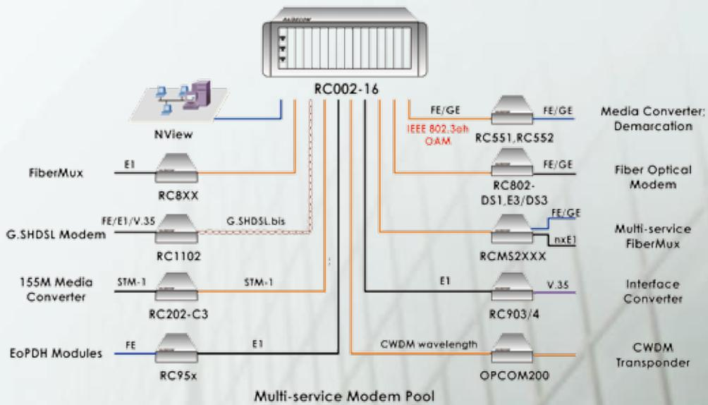
RC002-16 offers carriers a winning deployment strategy and supports a combination of Raisecom modular devices, including E1/V.35 fiber modem, G.SHDSL modem, E1 to V.35 interface converter, Ethernet media converter, STM-1 copper to fiber media converter, fiber optical modem, multi-service fiber mux, video optical multiplexer, and etc., to deliver
