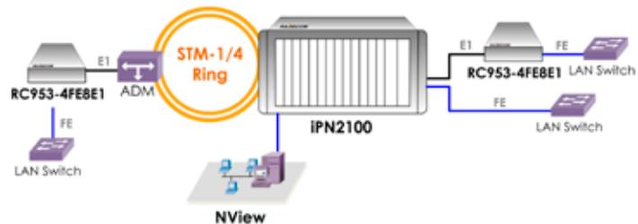
EOP-FEE1x8 tributary card encapsulates 8 Fast Ethernet into 8 VC12 respectively, providing 2Mbps bandwidth throughput on each link
