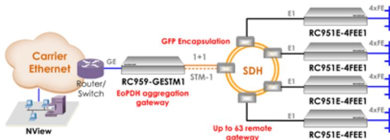
Working in point-to-multipoint topology with an EoPDH aggregation gateway
