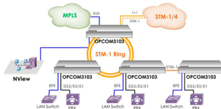
OPCOM3103 is deployed as an add & drop multiplexer (ADM) in a daisy chain
