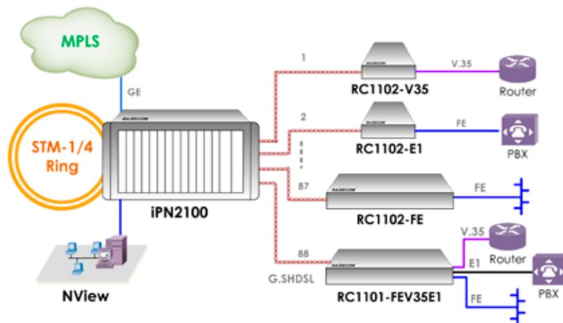
**Extending and aggregating E1, V.35 and Fast Ethernet services to STM-1/4 over multiple 2-wire copper cables**
