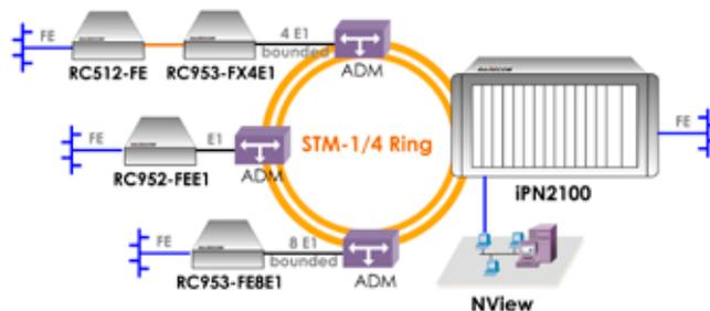
OPCOM3500E-EOP-FE16E1 aggregates Ethernet services through bonded VC12 (E1), and manages RC95x and RC512 converters remotely
