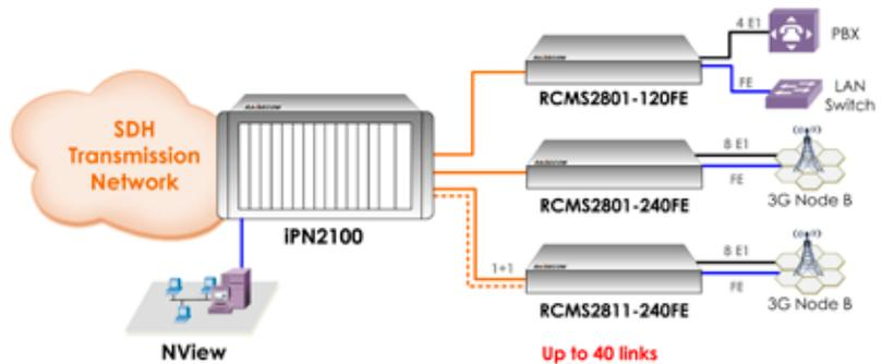
**Multi-service cards working with remote RCMS to deliver 1-8 E1s and aggregate wire-speed Fast Ethernet into SDH transportation**
