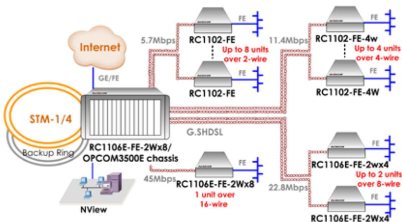
Aggregation fast Ethernet services to one GE/FE over cooper wire
