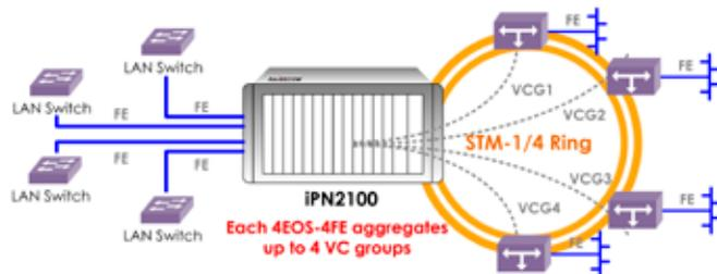
**OPCOM3500E-4EOS-4FE provides flexible switching between customers' Fast Ethernet services and the VC groups in SDH transportation**
