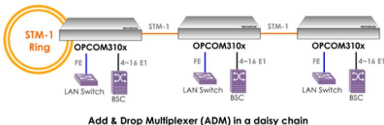
OPCOM3105 provides a fixed set of 4 E1 interfaces, 4 Fast Ethernet interfaces (over two VCGs), and 1 expansion E-SUBM slot with additional 2/4 E1, 1/2 V.35, or 1 Fast Ethernet over 1-4 E1 interfaces. OPCOM3107 has a fixed set of 8/16 balanced/unbalanced E1 interfaces, 4 Fast Ethernet over 2 VCGs, and dual redundant power supplies.
