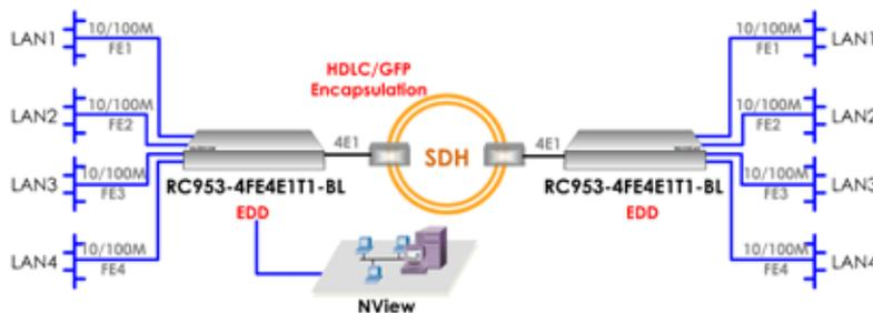
Point-to-point application of Ethernet Demarcation Devices with E1 uplinks
