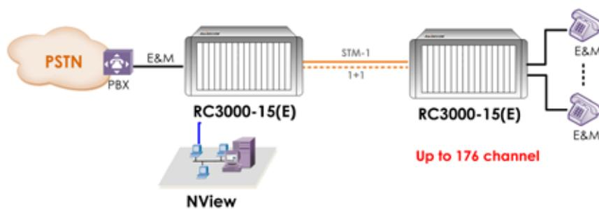
**E&M trunk lines application of Multi-Service Access Node**
