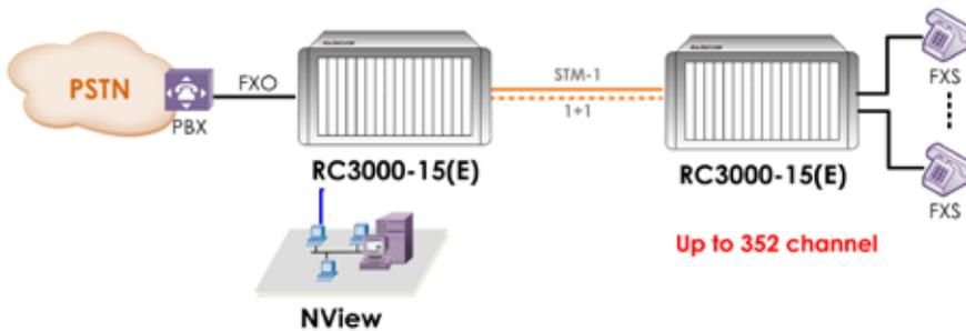
Loop signaling application of Multi-Service Access Node
