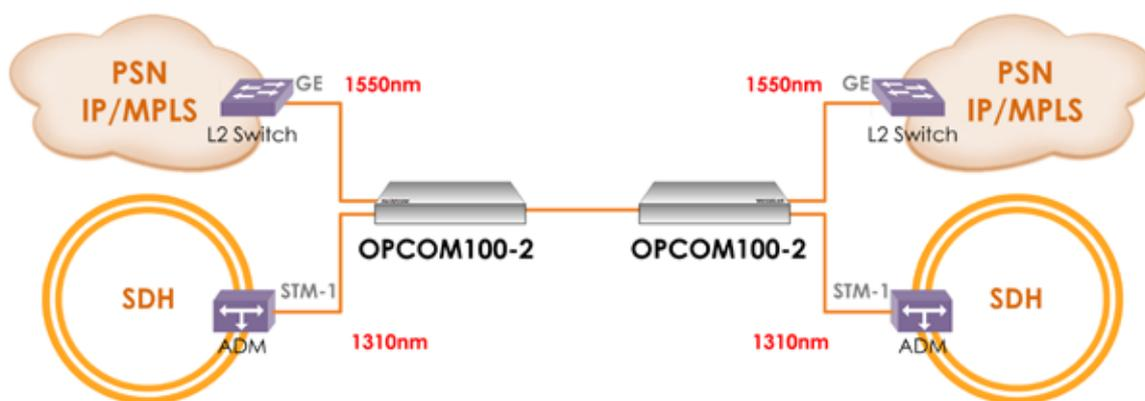
Point-to-point 2-channel CWDM solution
