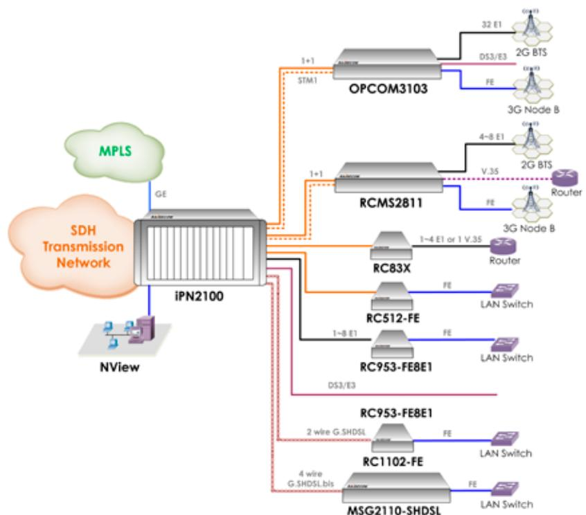
Aggregating various services via Raisecom CPE to STM-1/STM-4 and Gigabit Ethernet uplinks
