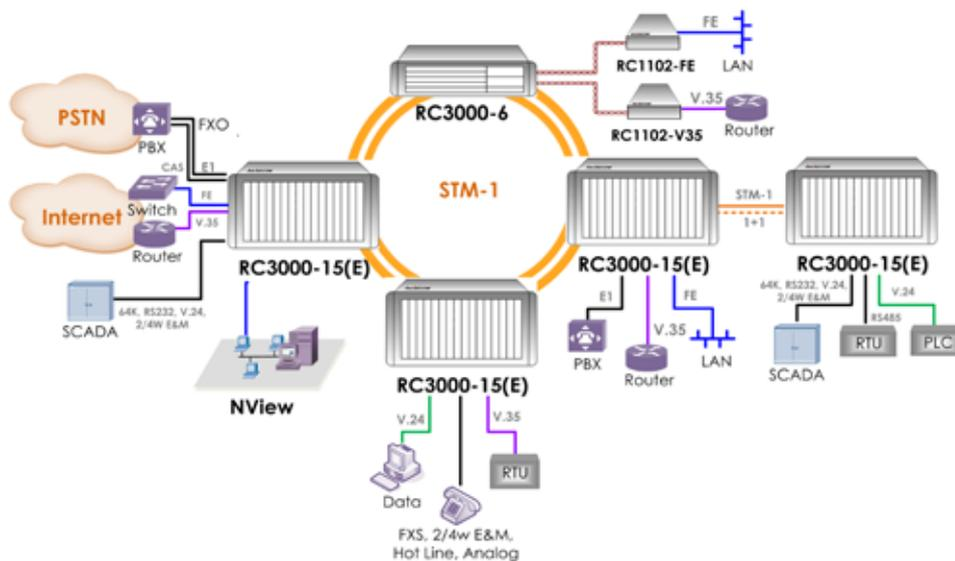
SCADA application of Multi Service Access Node
