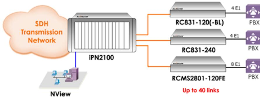
**MSAP provides fast and cost effective E1 extraction and extension from central office to multiple customer premise locations.**
