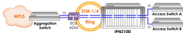
**OPCOM3500E-EOS-8FE provides max 80 ports of Fast Ethernet services over 4 STM-1/STM-4 uplinks**
